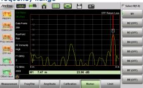
DTF is a way to locate faults identified by Return Loss or VSWR measurements.
