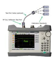
This calibration can be done either at the instrument test port, or at the end of a phase stable cable, in which case it compensates for the length of the cable. This is useful when measuring DTF. One side effect of the high accuracy OSL calibration is that it is dependent on the frequency span of the antenna tester. If the start and stop frequency is changed, the OSL cal will need to be redone.
